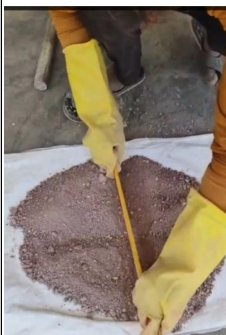
Photo No: 30 coning and Quartering
