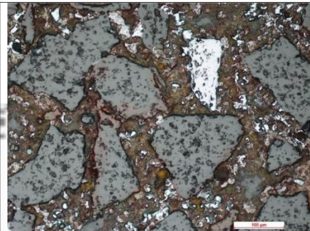
Fig. 3.7 Magnetite as detrital mineral; ferruginous cement; under reflected light
