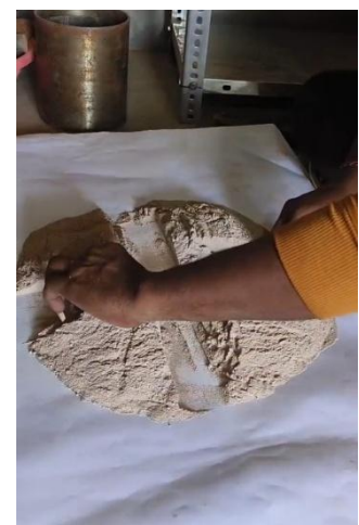
Photo No: 30 coning and Quartering
